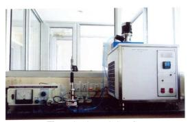
Figure 1. Ultrasonic interferometer
